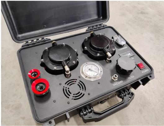
Quiet and easy to use while very effective at quickly removing unwanted air from the liner during the wet out process thanks to its high flow and vacuum suction.
